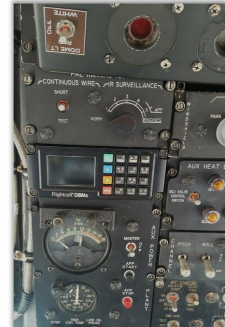
DZMx Installed in the Overhead Panel
