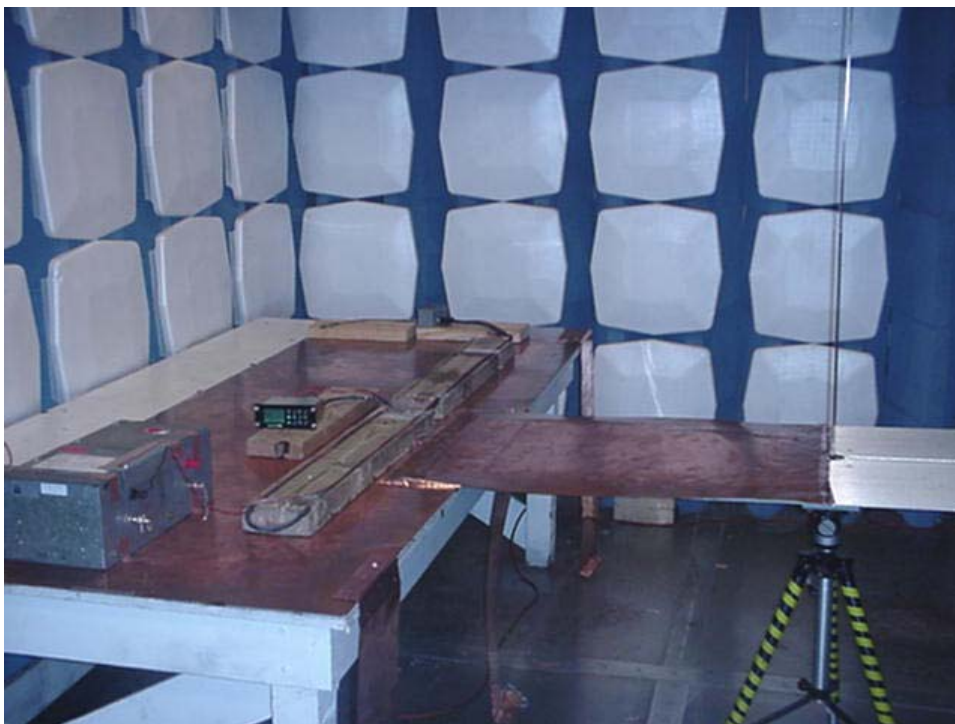
Photograph 3.1.8 Section 21 RE Rod Antenna – Side view
