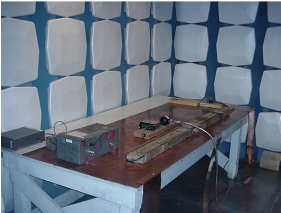
Photograph 3.2.2 Section 21 CE Test Setup – Side view
