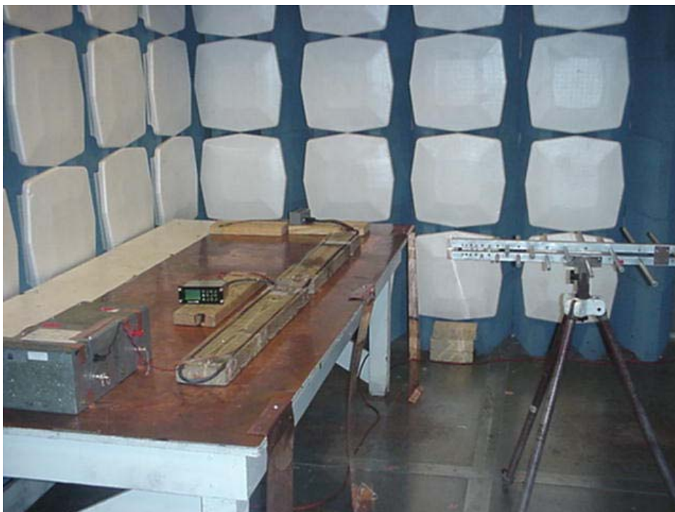
Photograph 3.1.6 Section 21 RE Log Antenna – Side view
