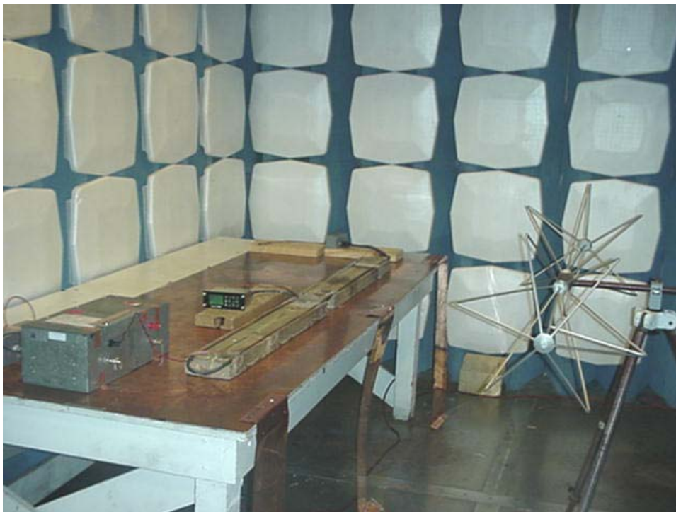
Photograph 3.1.2 Section 21 RE – Biconical Antenna – Side View
