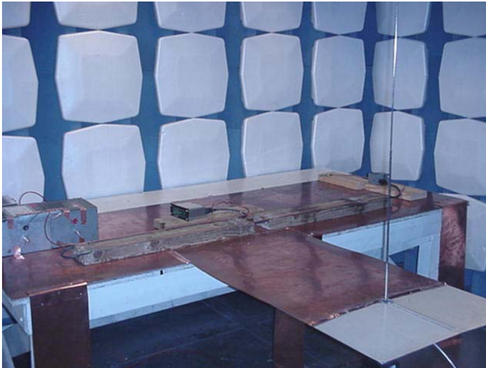
Photograph 3.1.7 Section 21 RE Rod Antenna – Test Setup
