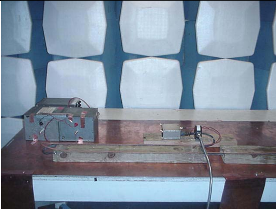
Photograph 3.2.1 Section 21 CE Test Setup
