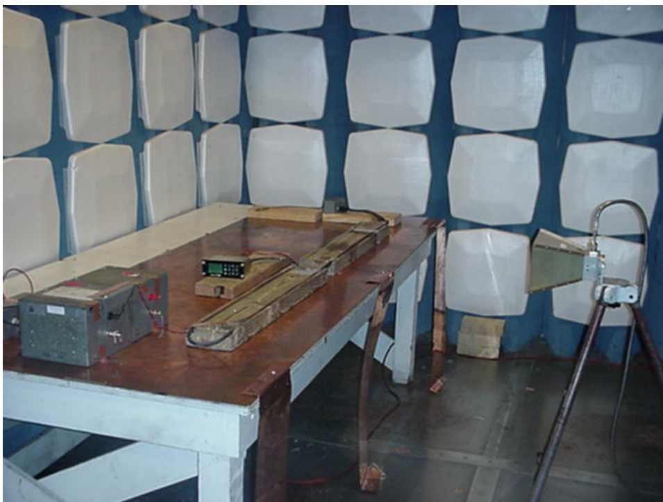
Photograph 3.1.4 Section 21 RE Horn Antenna – Side view
