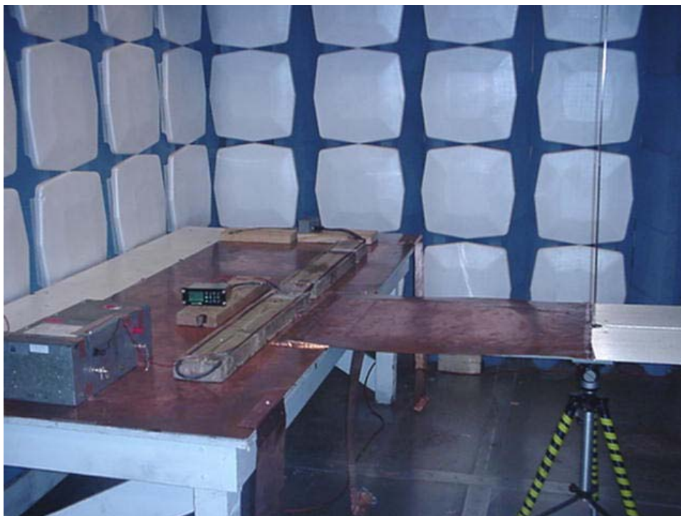
Photograph 3.1.8 Section 21 RE Rod Antenna – Side view
