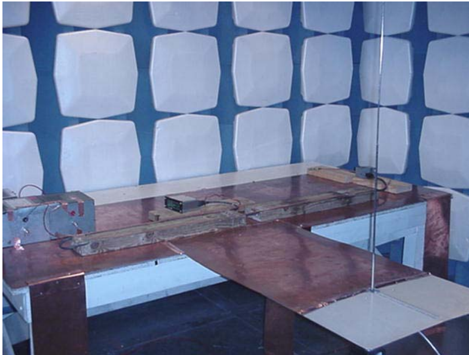
Photograph 3.1.7 Section 21 RE Rod Antenna – Test Setup
