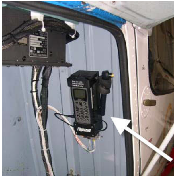
FIG: Iridium 9505A Phone Mount installed in side locker in Eurocopter AS350
