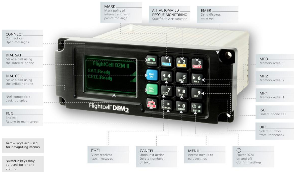
FIGURE 3: FRONT PANEL - ENGLISH CIVIL UNIT
