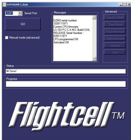
The firmware upgrade will normally take about a minute. The bootloader should now be running and the DZM display will show:
