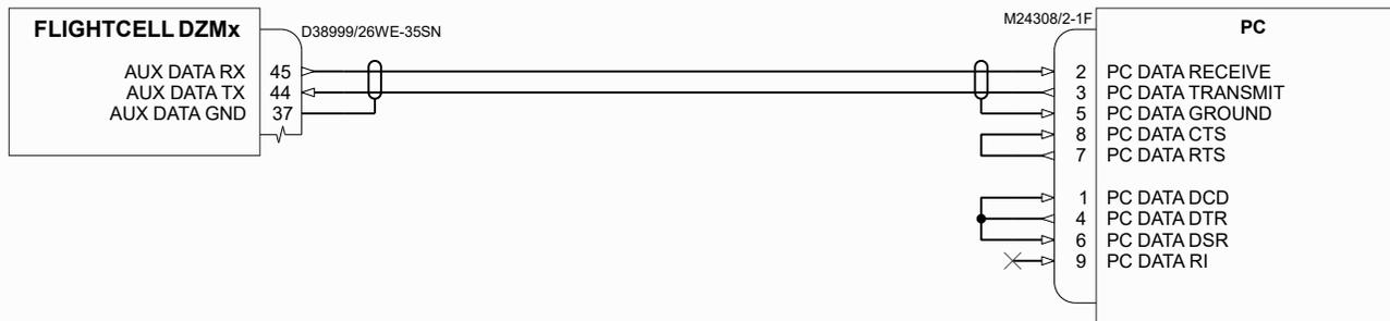
Note: the diagnostic port can be fitted for in-situ maintenance purposes. If fitted it is highly advisable to locate this connector such that it is readily accessible.
