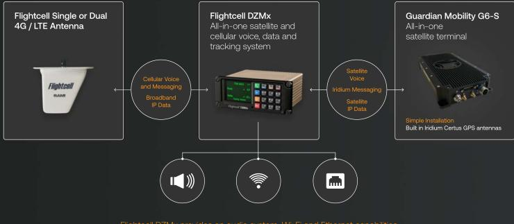
Flightcell DZMx provides an audio system, Wi-Fi and Ethernet capabilities
